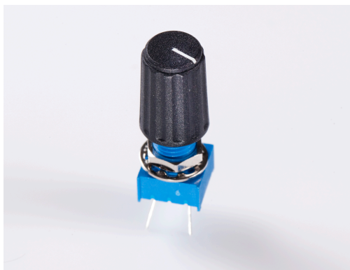
Figure 3-10. Potentiometers can measure rotation
