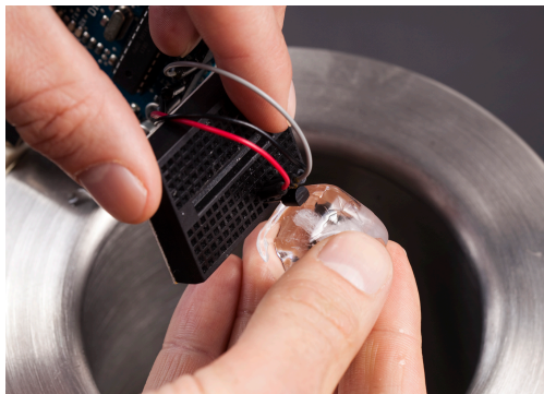
Figure 3-19. Testing the LM35 with an ice cube
